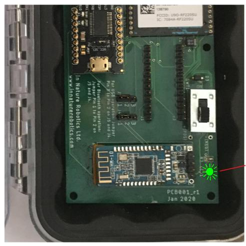
LED flashes at 1Hz rate when communications are ready (approx. 1 minute after powerup).
