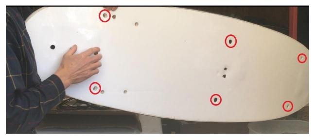
Use the two long plastic caps for the holes in the middle portion, where the foam of the boat is a bit thicker. Do not over-tighten the bolts; they should be just tight enough so that it is possible to swing the brackets back and forth with a bit of resistance from the foam of the surfboard.
